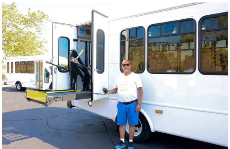
Armando, a driver for Renewing Life, demonstrates a wheelchair lift on one of their vans.
